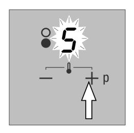
**3.** To change the heat setting: Touch the + or – symbol until the desired heat setting appears.
