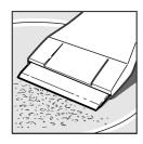
Remove the protective cover from the glass scraper. Only use the blade to clean the glass ceramic surface. The casing may scratch the ceramic surface.
