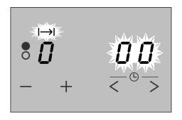
When the memory program has finished, the hotplate switches off. A signal sounds.  $\square\square$  flashes in the timer indicator. The  $\longrightarrow$  hotplate indicator flashes.  $\square$  lights up in the hotplate indicator.
