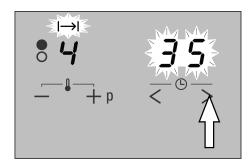
4. Touch the < or > symbol until the desired cooking time appears in the timer indicator. The cooking time flashes for several seconds and then disappears. If you have set a cooking time for several hotplates, it is always the shortest cooking time that is displayed. The I→I hotplate indicators light up.
