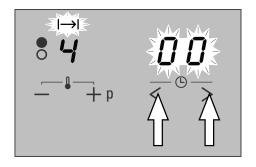
You enter a specific cooking time for the desired hotplate. When the cooking time has elapsed, the hotplate switches off automatically.
