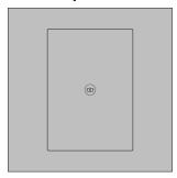
The plate—warming zone is used for melting chocolate or butter, and for keepingplates and receptacles hot. Do not use aluminium foil or plastic, as it will melt.
